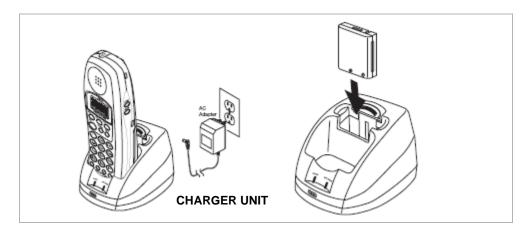
NOTE -- A flashing LED on the charger indicates the handset is not seated properly, the battery is not hooked up, or the telephone is not in service.
