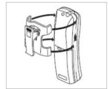
3. Press firmly until the belt clip snaps into place.
